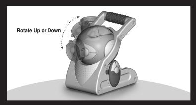
**3.** Grasp the focus ring and rotate to adjust the height of the projected image.
